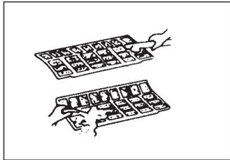
5. Install the air freshening filter back into position.
